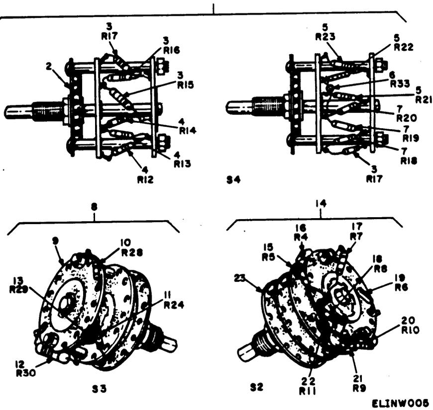
Figure 5. Switch assemblies.
